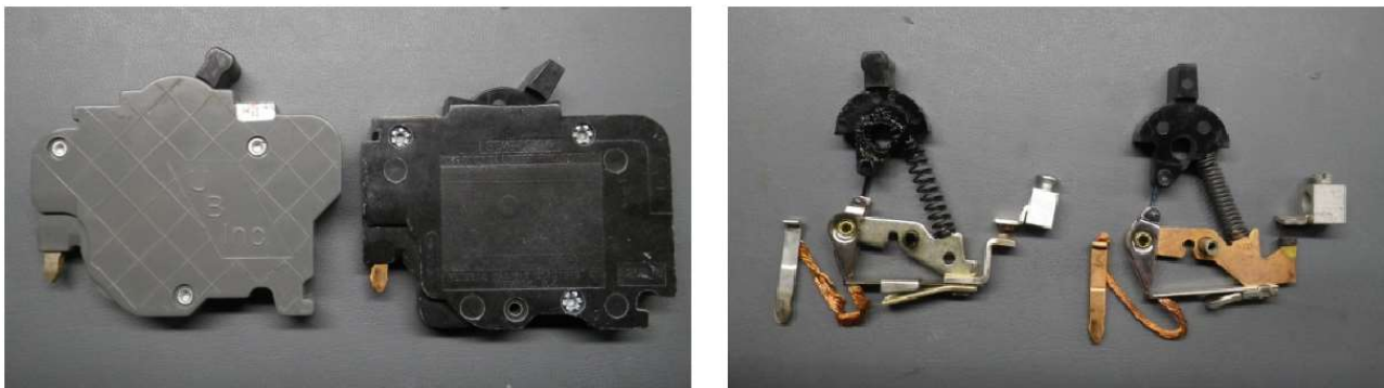
FIGURE 13 - UBI-F BREAKER AND FPE BREAKER, OUTSIDE AND INSIDE (UBI on left, FPE on right in both photos)
