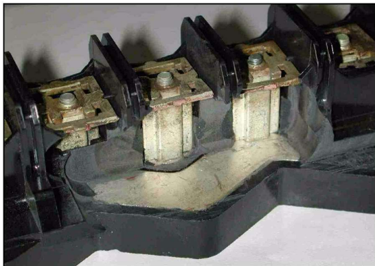
A. Cutaway - Bussbar, Post, and Stab Socket Plate.
